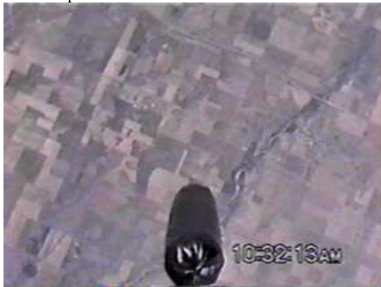
Figure 8. The Inflated Experimental Black Polyethylene Balloon Above the Colorado Plains
