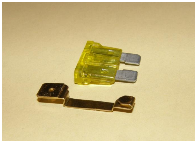
Figure 1 – Old style slip on auto fuse tap in front of an ATC style fuse
